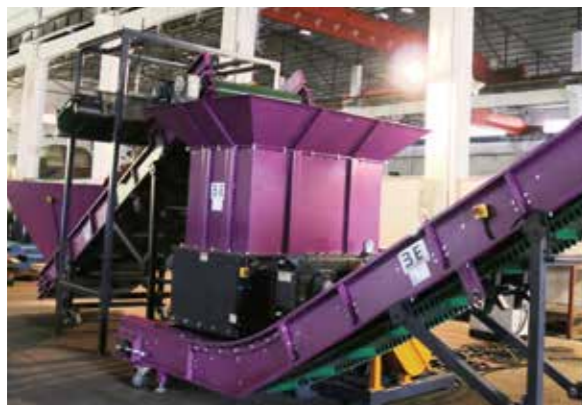
单轴 shredder WTF40120 配磁选生产线 Single shaft shredder WTF40120 with magnetic separation
