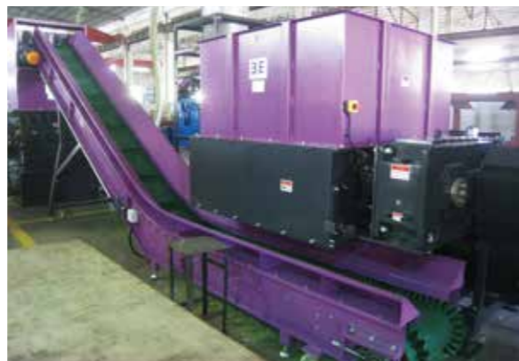
单轴 shredder WT40150 + 破碎机 PC52120 生产线 Single shaft shredder WT40150 with Granulator PC52120
