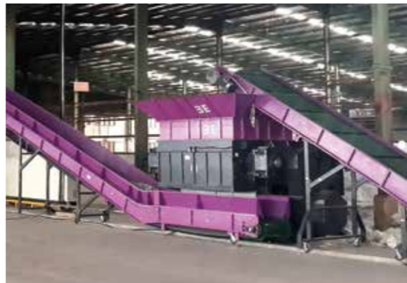
塑料破碎清洗回收线 Plastic crushing & washing line
