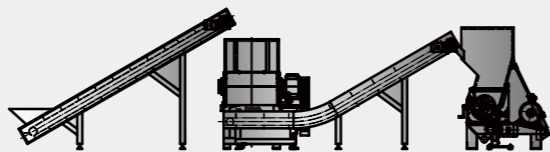
单轴撕碎机WT40100配破碎机PC4280 Single shaft shredder WT40100 with Granulator PC4280
